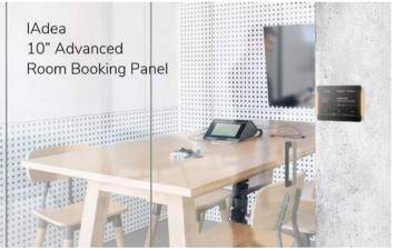
Furthermore, specially designed room booking panels provide bright colored lights on the sides of the screen, to extend the visible distance of room availability information. A green glow would indicate that the room is vacant, and red that the room is in session. Other uses of the light may indicate that a meeting is about to start (so don't take this room if the conversation will be longer than a few minutes),
